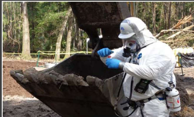
PBA TCRA – Excavation boundary sampling (8-25-14).
